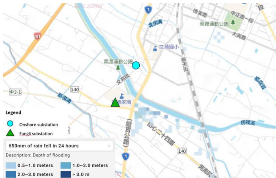
Figure 4.4: Hazard map showing areas with potential flooding (inundation height) from a 24-hour cumulative rainfall of 650mm
