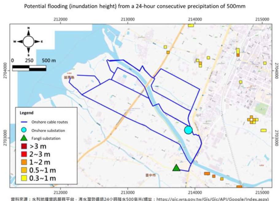
Figure 4.3: Hazard map showing areas with potential flooding (inundation height) from a 24-hour cumulative rainfall of 500mm
